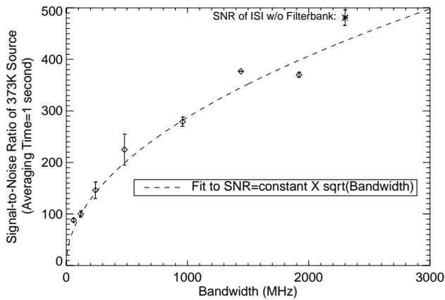
FIG. 5.—Plot of S/N for observations of a 373 K blackbody with and without the filter bank. This confirms that the system is shot noise limited and that the filter bank degrades the sensitivity by about 10% as expected.
