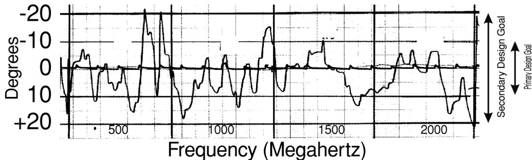
FIG. 4.—Relative phase response of the two filter-bank modules as a function of frequency. The bandpasses are matched to within  $10^\circ$  over 80% of the bandwidth and always within  $20^\circ$ .
