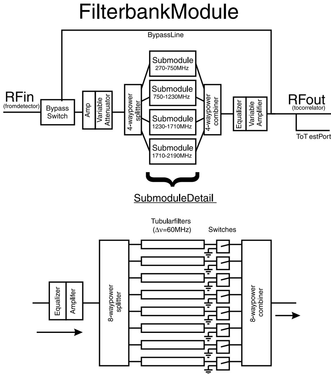
FIG. 2.—Block diagram of one of the filter-bank modules; there is one per telescope
