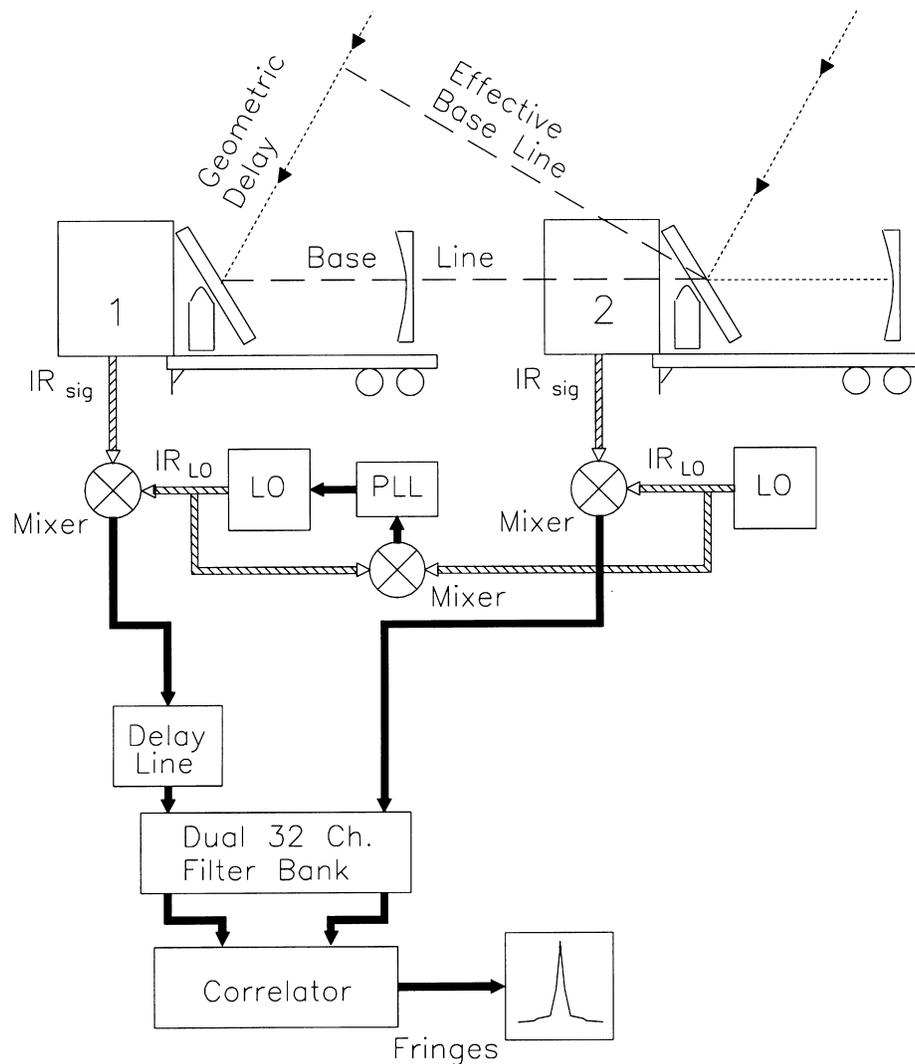
FIG. 1.—Block diagram of the ISI interferometer with the filter bank in the RF path. Two trailers, each containing a telescope, are indicated. IR signals are mixed with LO power from CO<sub>2</sub> lasers. After passing through a filter bank that determines the bandpass, the resulting RF signals from the two telescopes interfere in a correlator, producing interference fringes. The two LOs are kept in phase by a phase lock loop circuit. See Hale et al. (2000) for complete details.
